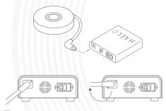
Carefully insert coil into the device, turn clockwise until the connector clicks into place. To remove, slide the silver button toward you and turn the connector counterclockwise.
